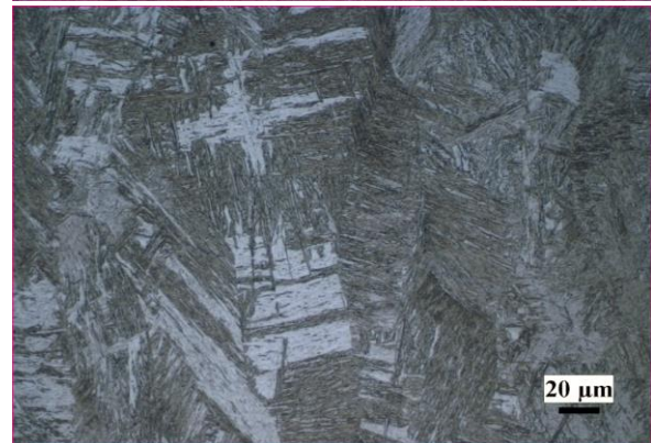
Figure 4. 500X 8kA – 20 cycle sample; a) weld button and HAZ b) welding metal.
