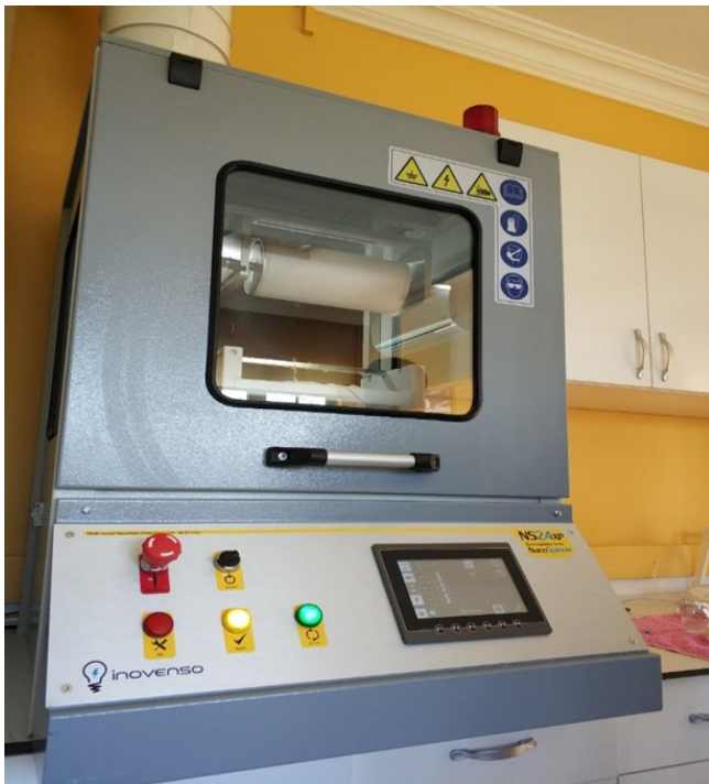
Figure 2.3. Electrospinning device used in the production of nano biocomposites (Inovenso NS 24XP, Turkey)
